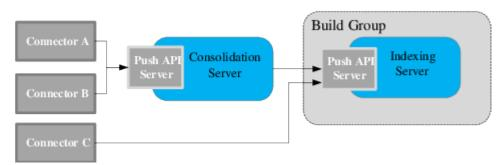
The following diagram illustrates the consolidation workflow within the Consolidation Server, when connectors push documents.
