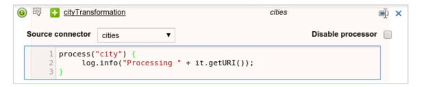
Although it is not explicitly visible in the method signature, the process method receives the current document being processed (transformation or aggregation) using the special it variable. You can see it in the above example with it.getUri(), which is the equivalent of IConsolidationDocument.getUri().
